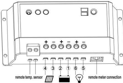
**Connect the individual components to the symbols provided, they are solar panel, battery and loads in order indicated 1-6.**
