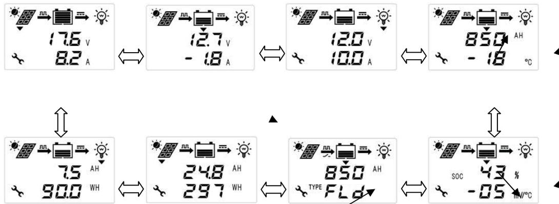
The data can be adjusted: battery capacity AH, battery temp. compensation, battery type. On read status, press K1/SET for setting data.
