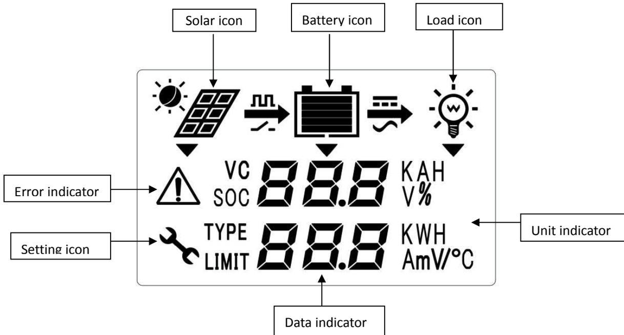
Two LED indicator above LCD, green on when charging. Yellow on when error.
